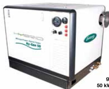
**WhisperPower's 50kW Genverter offers a new way of generating power – a variable-speed, ultra-compact and lightweight diesel generator (cont. power 50 kW/ 1200-3600 rpm/ fly wheel integrated AC alternator, based on Steyr 4 cyl engine).**
