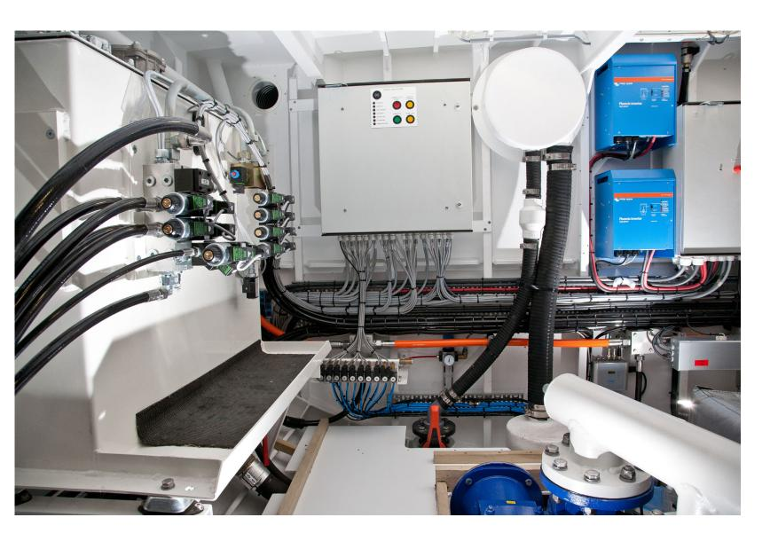
The technical systems are very advanced. The main engine is a Steyr 6-cylinder driving a folding propeller, while a 4-cylinder Steyr engine drives the integrated fly wheel generator (generating 4kW to charge batteries) and a hydraulic pump.
